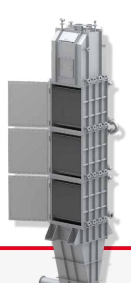
The deep knowledge of condensation phenomena and of the hygroscopic characteristics of the products allows FIC to design its own BSHE for fertilizers so that the condensation is always avoided, keeping the operating temperature conditions on the plate surface always above the dew point . This result is obtained thanks particulary to:
